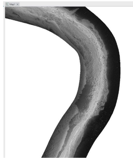
Figure 5 - Sonar mosaic with the water column removed (i.e. slant-range corrected)
